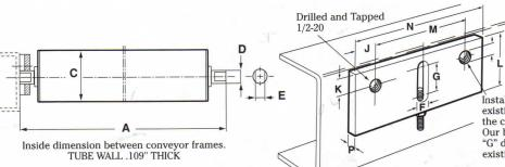
Dimensions shown are for our standard 4" c/c mounting bracket #13012. Optional 3" and 6" brackets are listed below:
